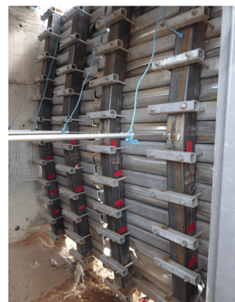
Figure 3: Square CFDST columns after air-blast loading
