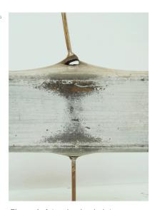
Figure 4: A tension-loaded, transverse branch plate connection exhibiting three failure mechanisms: (i) *Plastification of the HSS face*; (ii) *Punching shear of the HSS connecting face*; (iii) *Local yielding of HSS side walls*
