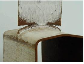
Figure 2: A heavily welded, tension-loaded, transverse branch plate connection (with B=1.0 and high  $\beta$ /t) demonstrating local failure of the branch plate. The parts of the plate width that are effective are illustrated by the two outer brown regions where the white-wash has flaked off.
