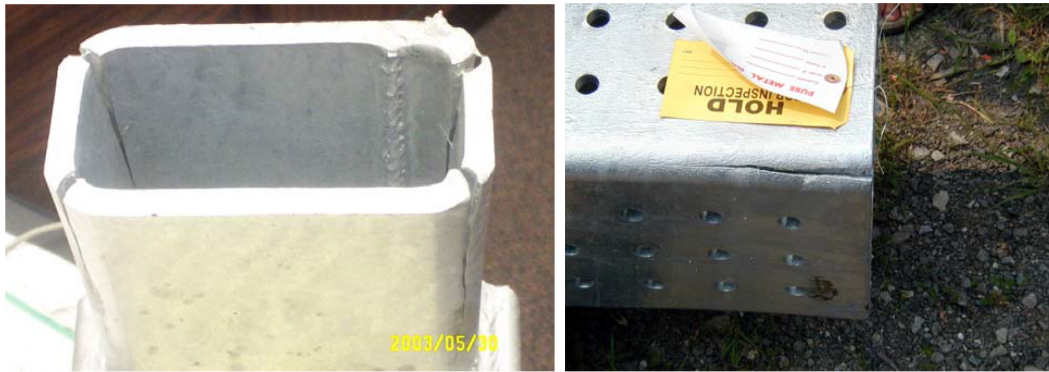
Figure 2: Examples of corner cracking in square and rectangular HSS, during hot-dip galvanizing
