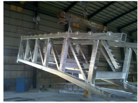
Figure 1: Segment of a HSS pedestrian bridge truss, after hot-dip galvanizing (Photo courtesy of American Galvanizers Association)
