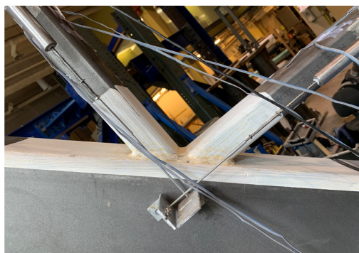
Figure 3: Testing arrangement for isolated zero-gap K-connections
