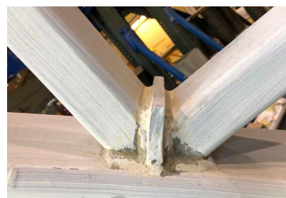
Figure 2: Use of a vertical division plate between the two branches
