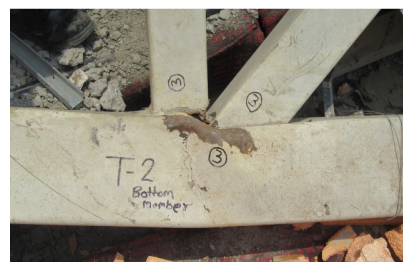
(b) In-service connection failure Figure 1: Rectangular HSS K- (or N-) connections with zero gap between the toes of the branches
