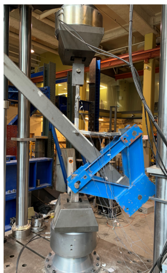
Figure 3: Testing arrangement for isolated zero-gap K-connections
